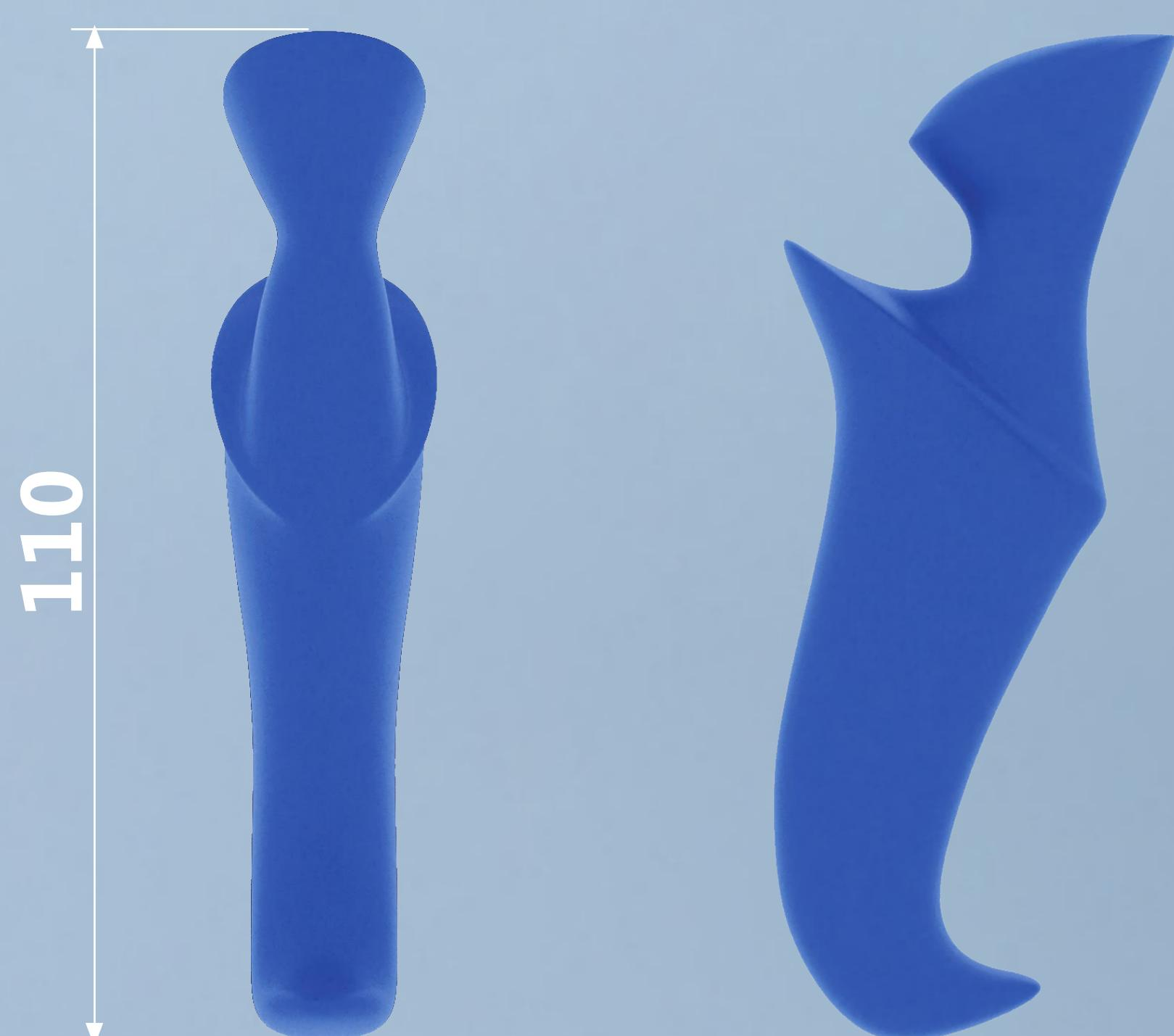
The goal of the handle design is to guide a person, to hold the goldsmith's saw correctly in a way that reduces the number cracked slices.
